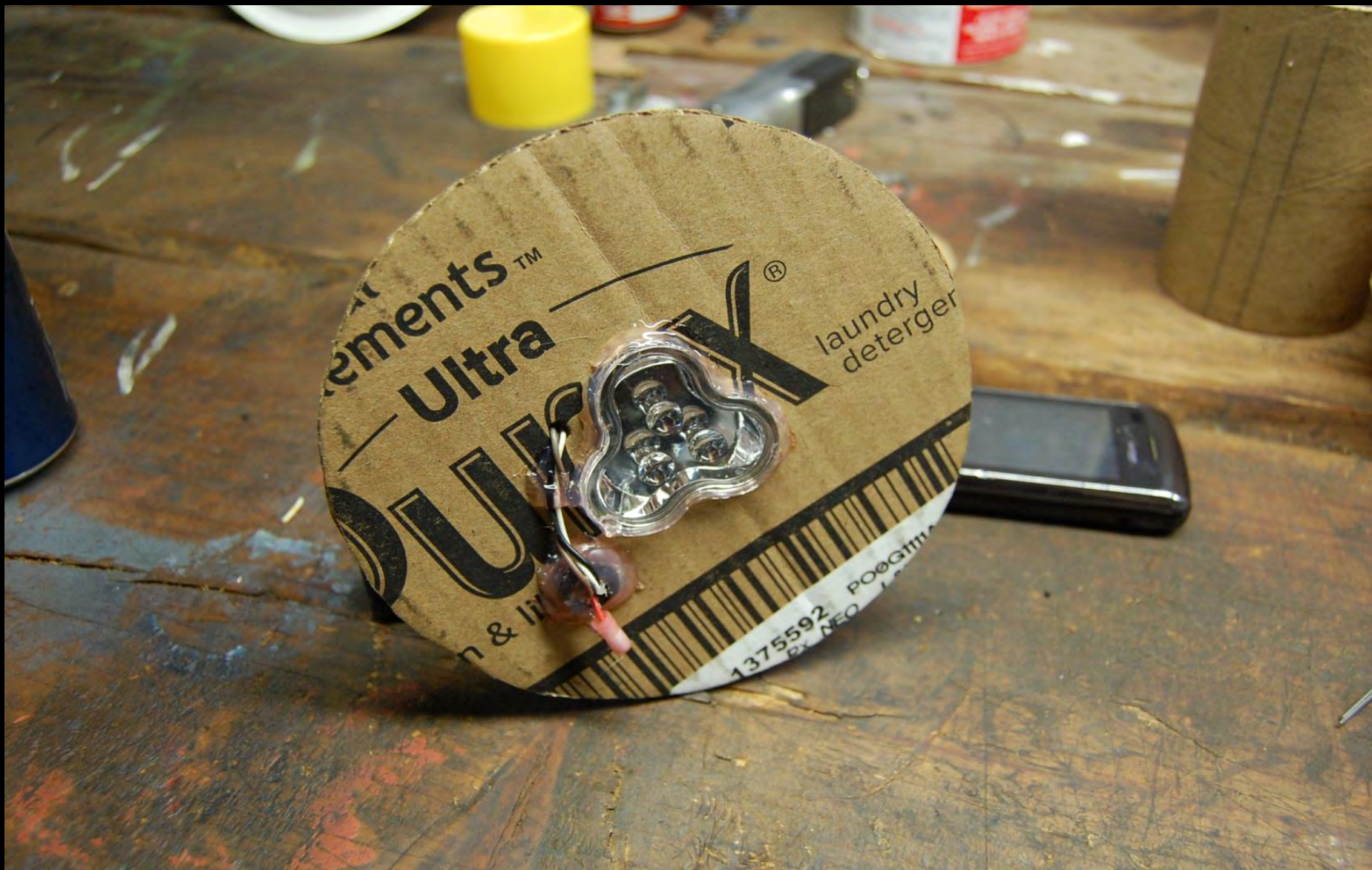
(November, 2010) I constructed our very first indoor light trap using three magnified LED lights.
